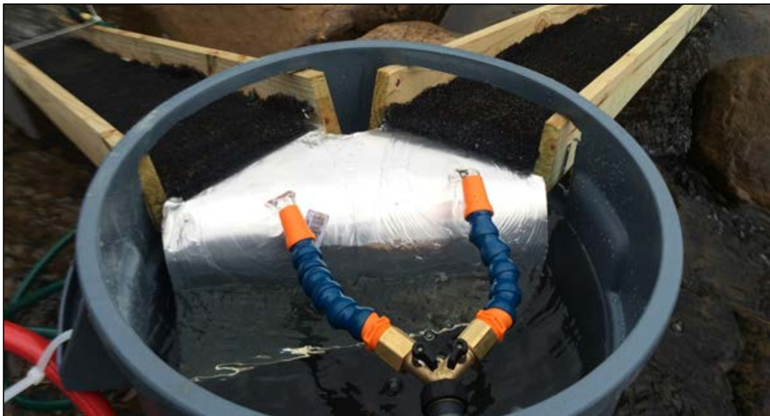
PHOTO 4 NOZZLE SETUP FOR PROVIDING FLOWS ONTO RAMPS
