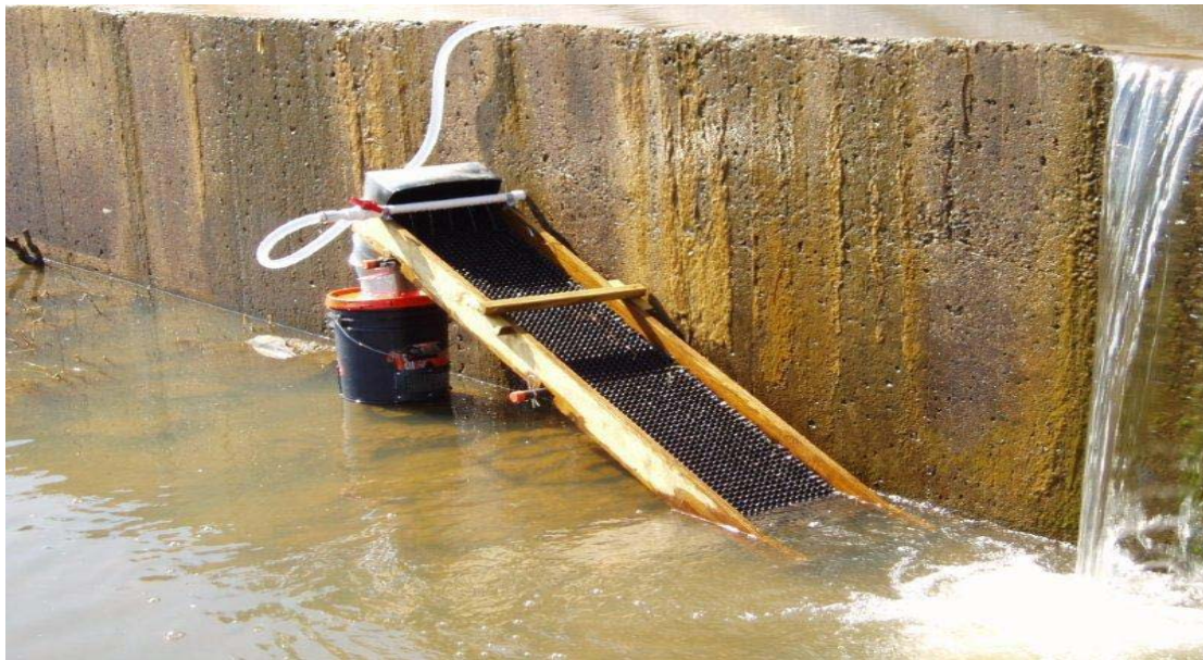
FIGURE 2. EXAMPLE OF A PORTABLE ELVER RAMP TRAP USED AT THE DOMINION PROJECT TAILRACE.
