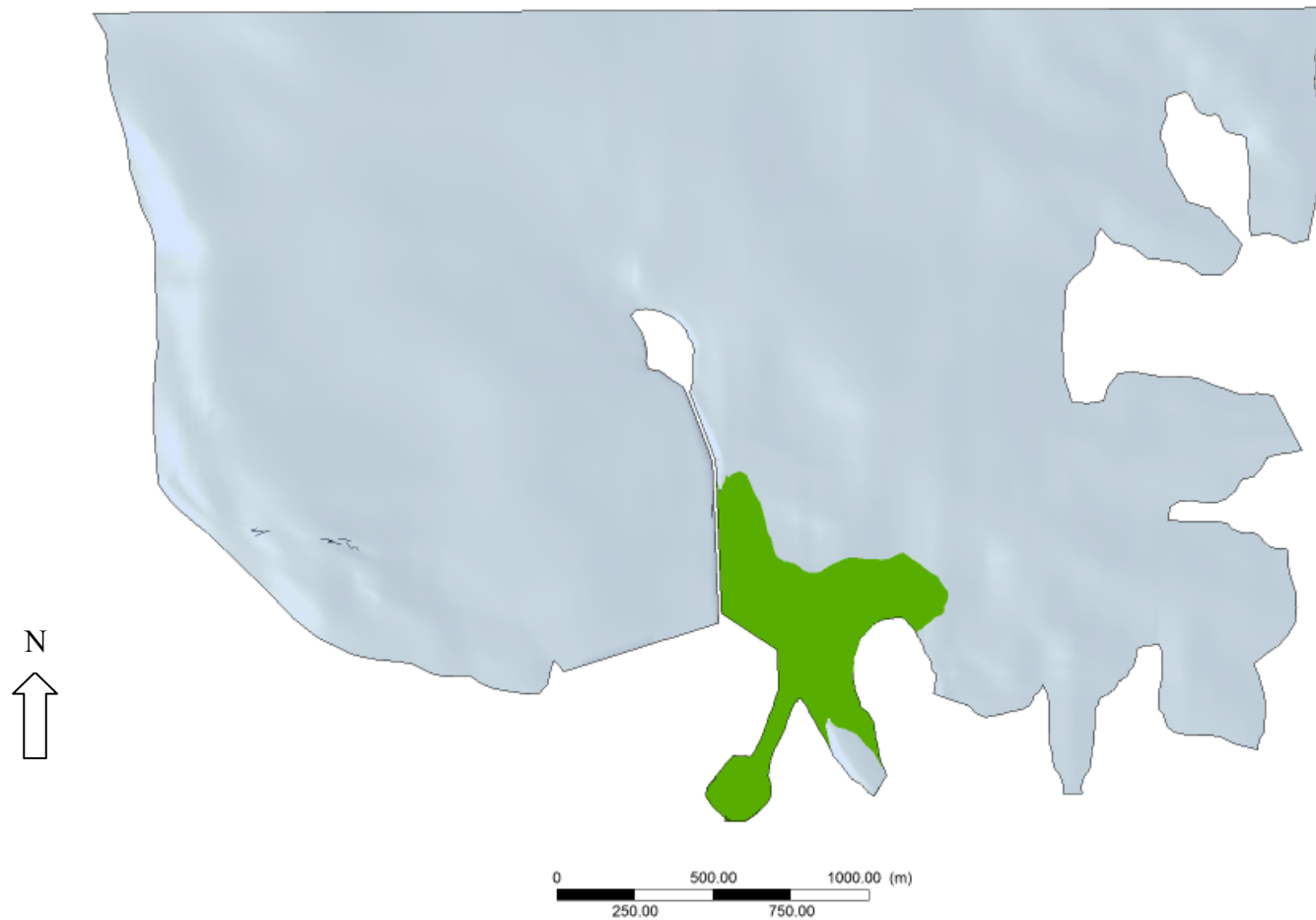
Figure 27 – Scenario 1W, \Delta T = 5^{\circ}\text{F} thermal plume (green).
